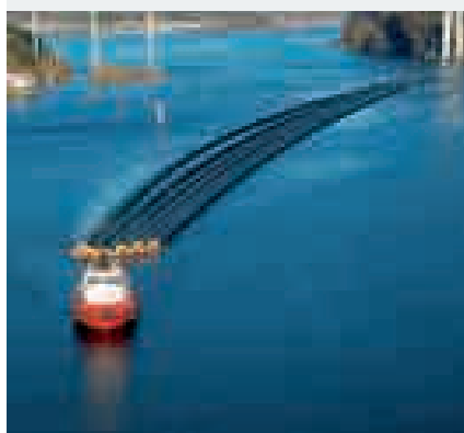
Pictured: Storm overflow pipes travelling from Norway to Anchorsholme to be used as part of our bathing water quality programme.
